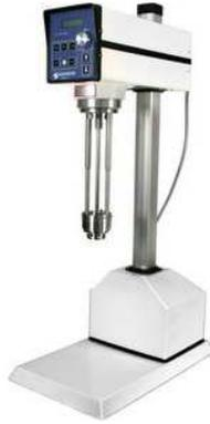
**Figure 1 Silverson high shear mixer used for production of graphene in [2]**
