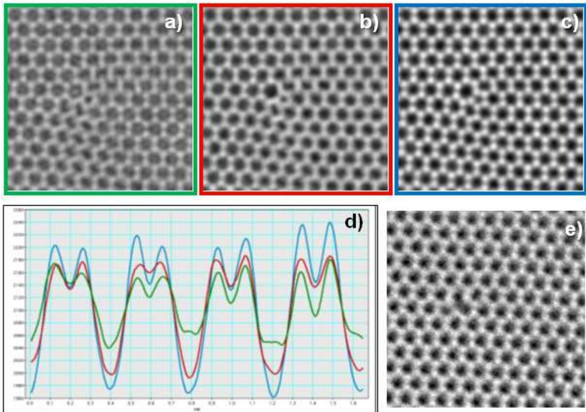
Fig.1. Simulation verification of the impact of optimum conditions: a) Scherzer conditions optimized for 0.1 nm transfer; b) C5+C3+df conditions optimized for 0.1 nm transfer; c) C5+C3+df conditions optimized for 0.1 nm transfer and systematic error from Zemlin tableau is accounted; d) the intensity profiles across simulated images; e) an experimental image acquired at approximately optimum conditions.
