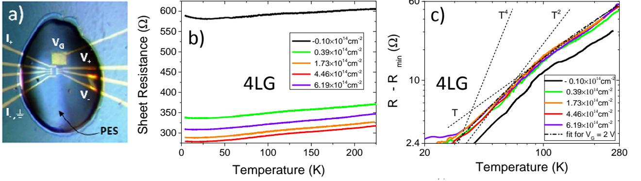
Figure 1: a) Micrograph of one of the FLG devices; b) T dependence of the sheet resistance at different gating-induced surface charge densities in a 4LG device for electron doping; c) Log-log plot of the increase of the sheet resistance in the range 20–280 K for the same 4LG device
