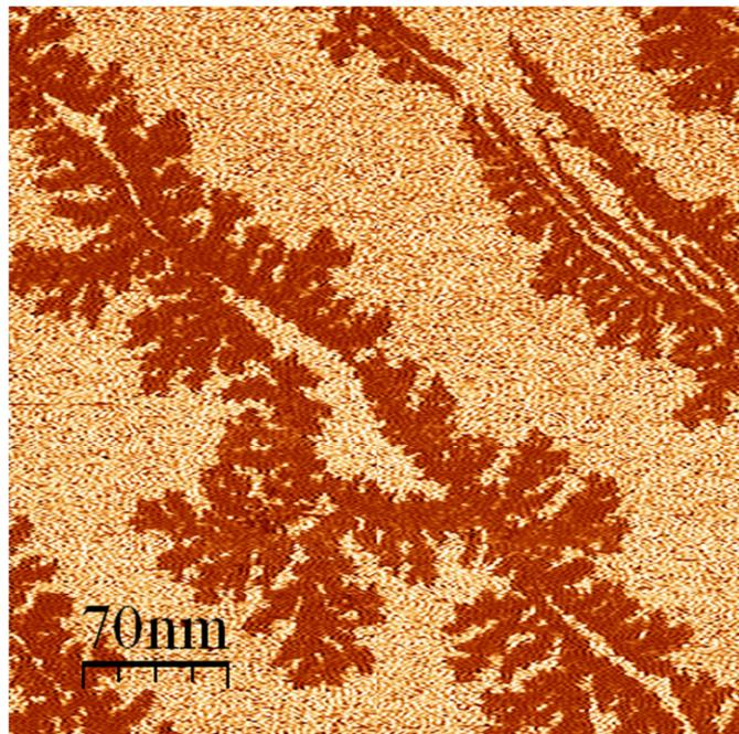
Figure 2: Current STM image of graphene on Au(111) showing long dendritic. Graphene appears as darker areas in this type of pictures (Bias Voltage = -1241.7mV, Current set-point = 0.04nA).
