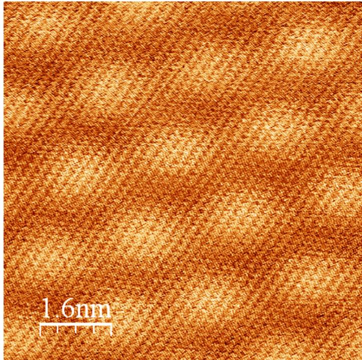
Figure 1: STM image of graphene on Pt(111) showing a long range moiré pattern and atomic resolution (Bias Voltage = -35.7mV, Current set-point = 0.04nA).
