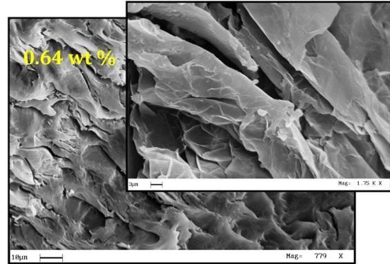
Fig.2: SEM images of the fracture surface of composites filled with 0.64 wt% of exfoliated graphite.
