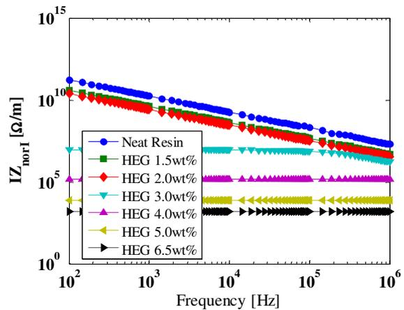
Figure 4: AC behavior of the nanocomposites in the frequency range 100Hz-1MHz. Impedance magnitude normalized with respect to material thickness.
