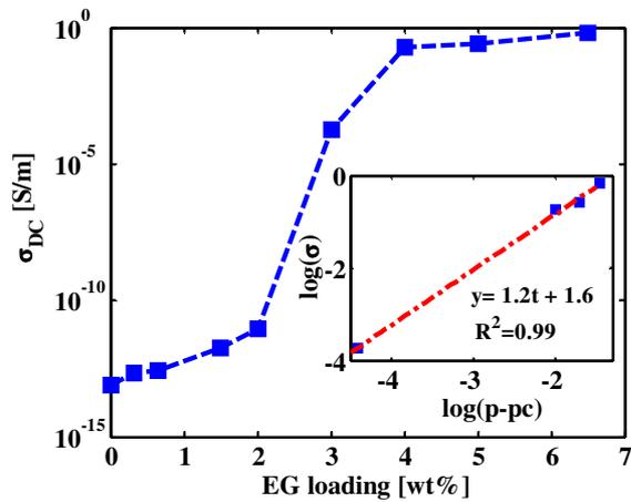
Figure 3: DC volume conductivity of the nanocomposites versus CNFs weight percentage. The inset shows the log-log plot of the electrical conductivity as a function of (p-pc) with a linear fit.
