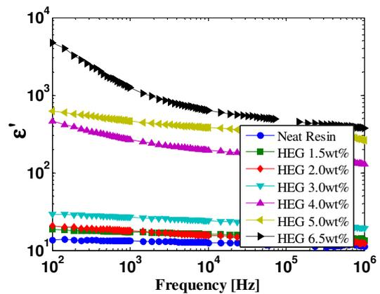
Figure 6: Dielectric permittivity of composites with different EG content as function of frequency
