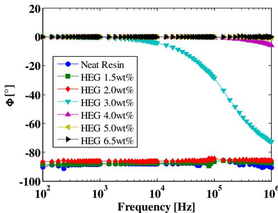
Figure 5: AC behaviour of the nanocomposites in the frequency range 100Hz-1MHz: Phase in degrees.
