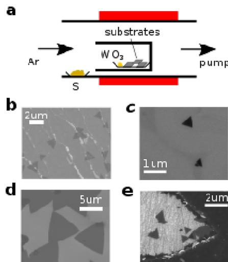
**Fig. 1 | Simultaneous CVD growth of WS<sub>2</sub> on various substrates.**
