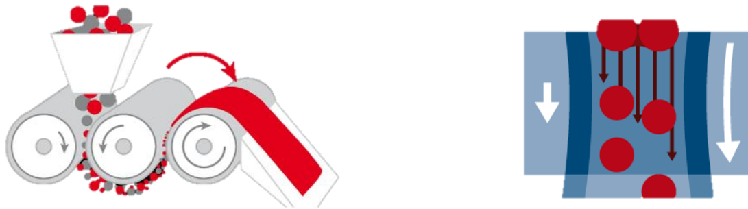
Figure 1: The three roll mill mechanism.
