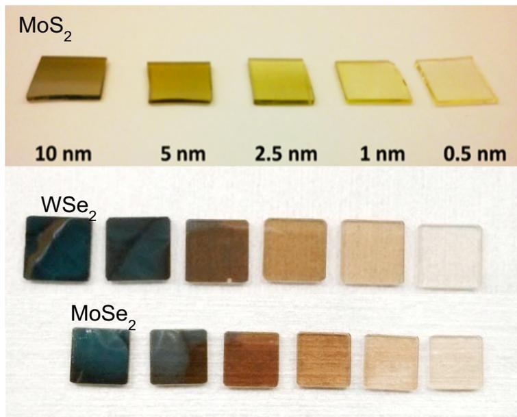
Figure 1: Synthesized TMD films on the quartz substrates show different transparency depending on film thickness.
