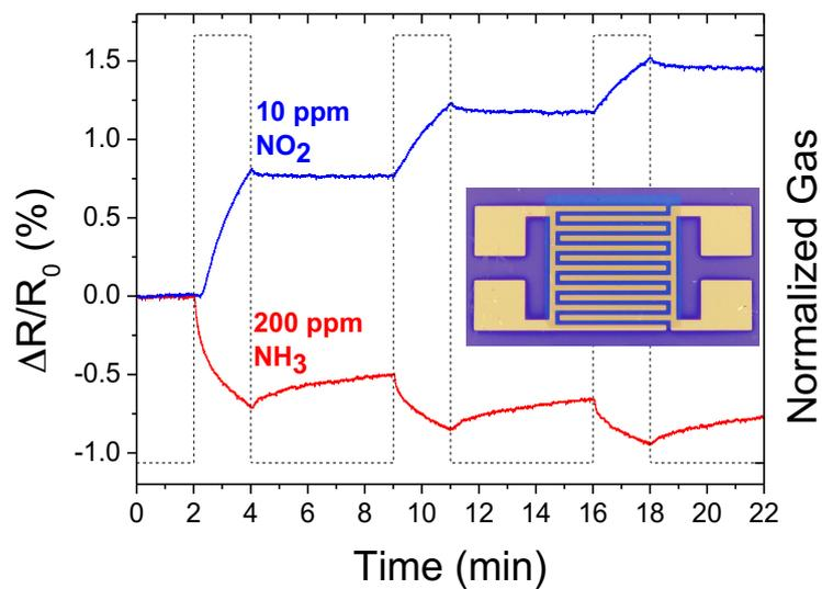
Figure 2: Sensor response curves of the MoSe<sub>2</sub> sensor at 10 ppm of NO<sub>2</sub> and 200 ppm of NH<sub>3</sub> gases, respectively. Inset: Photograph of a contacted MoSe<sub>2</sub> sensor.
