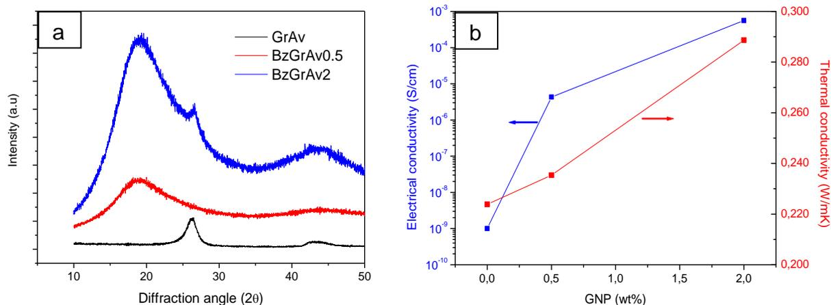
Figure 1: (a) Diffraction patterns of graphene and nanocomposites with a 0.5 and 2 wt.% of GNP; (b) Electrical and thermal conductivity of benzoxazine and its nanocomposites.
