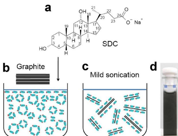
Figure 1: Graphite exfoliation. (a) Molecular structure of SDC. (b) Schematic illustration of the graphite exfoliation process. (c) A mild ultrasonication produces exfoliated mono- and few-layer graphene encapsulated by SDC. (d) Photograph of the as-prepared dispersion.
