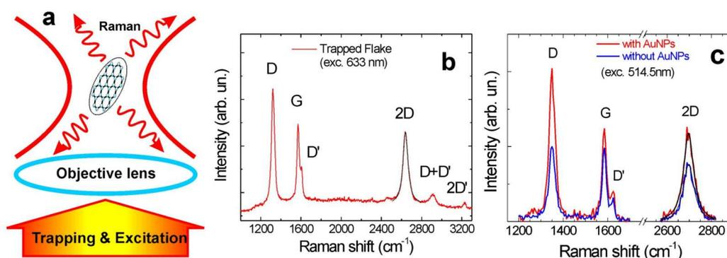
Figure 2: (a) Experimental setup. The same optics is used to trap graphene in dispersion and collect the Raman signal that is sent to a spectrometer. (b) Raman spectrum of an optically trapped flake for 633 nm trapping and excitation wavelength. (c) Micro-Raman spectra of graphene dispersions with and without gold nanoparticles for 514.5nm excitation.
